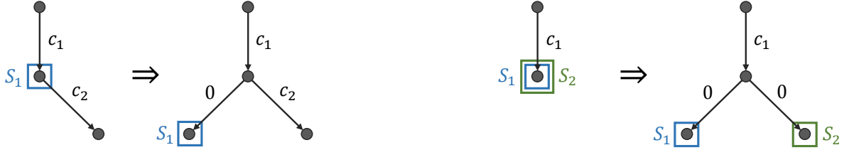
Figure 2: Examples of reductive equivalence transformations. On the left, a non-leaf vertex is pulled out to a leaf in order to ensure that all vertices belonging to sets are leaf vertices. On the right, a vertex contained in two sets is split into two new vertices to ensure that all vertices belong to at most one set. Both transformations preserve the optimal solution.
